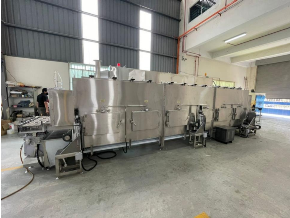
Figure 1 Clean Room Hard Disk Drive Curing Conveyor Oven
